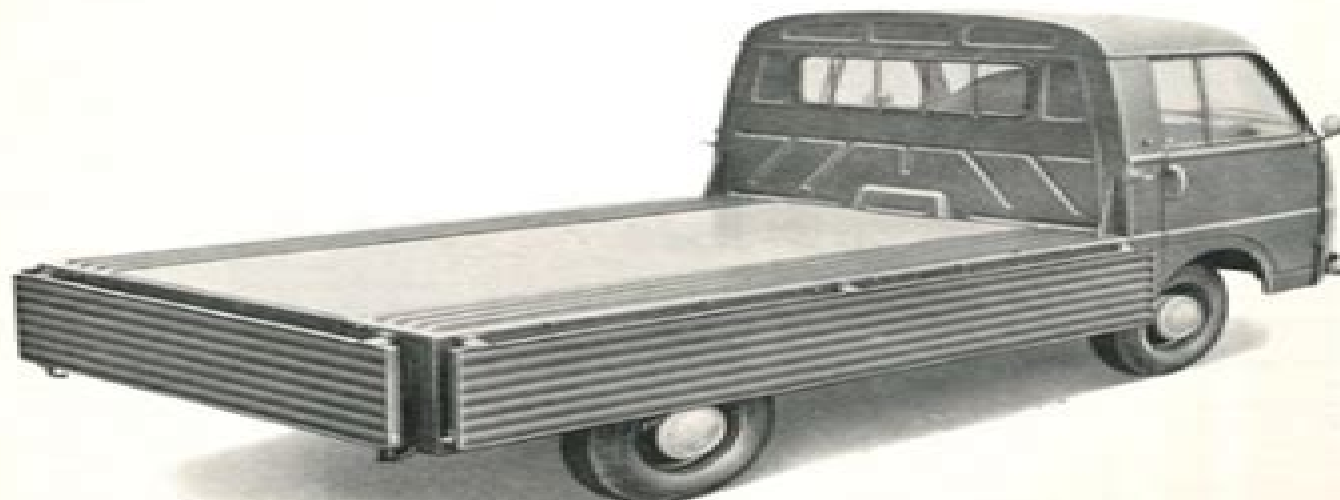
Fig. 1. Three-quarter rear view of the pickup model 1100 T (type 257 D), with the side and rear panels dropped.
