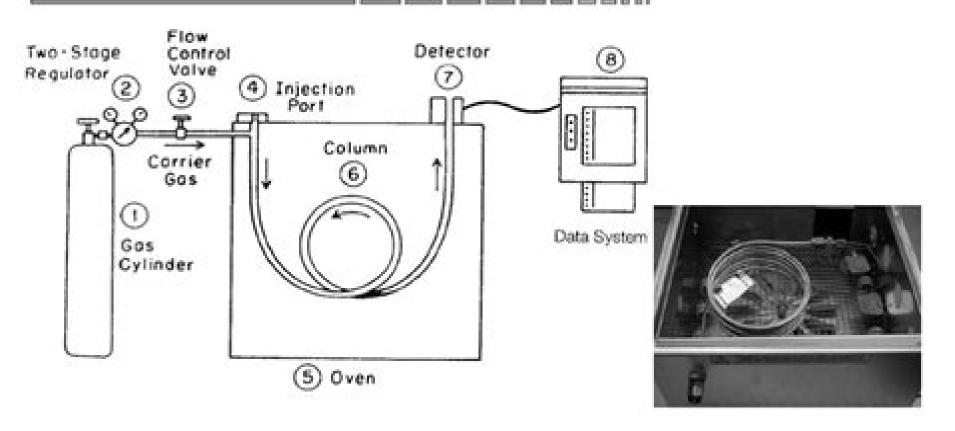
Schematic diagram for gas chromatograph
